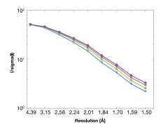
Figure 1: Fine φ-slicing with PILATUS. Each data set was collected at the same angular speed of 0.1 °/s in only 30 minutes with decreasing rotation width and exposure time per image as indicated in the legend. Excellent data are obtained with short acquisition times. Exploiting fine-sliced data collection with a noise-free PILATUS leads to optimal data quality (insulin, 180° total rotation, microfocus sealed tube, PILATUS 300K).
