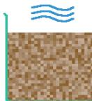
Dry the sample until still moist, ~15% water content. Gentle warming can be used to accelerate the process, but take care not to over-dry in places, and allow time for the water content to equilibrate throughout the sample before taking a reading.
