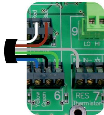
In DeltaLINK<sup>4</sup> configure channel 6 as type **ML3** and channel 7 as a type **ML3 Temperature** sensor.
