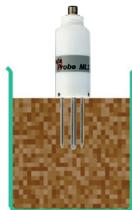
Insert ML3 into the wet sample and record its output in Volts.
