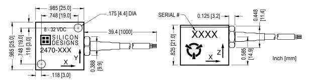
Note: The cable's braided shield is electrically connected to the case. The black ground (GND) wire is isolated from the case.
