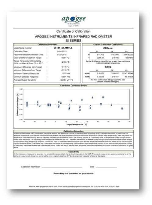
Calibration overview data are listed in box in upper left-hand corner, sensor specific calibration coefficients are listed in box in upper right-hand corner, temperature errors are shown in graph, and calibration date is listed below descriptions of calibration procedure and traceability.
