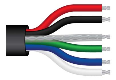
Red: High side of differential channel (positive thermopile lead)
