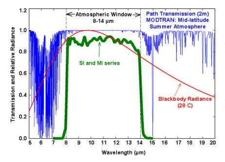
Spectral response of SI series infrared radiometers. Spectral response (green line) is determined by the germanium filter and corresponds closely to the atmospheric window of 8-14 µm, minimizing interference from atmospheric absorption/emission bands (blue line) below 8 m and above 14 µm. Typical terrestrial surfaces have temperatures that yield maximum radiation emission within the atmospheric window, as shown by the blackbody curve for a radiator at 28 C (red line).
