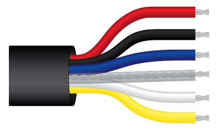
Red: Power In (4.5-24 V DC) Black: Ground (for sensor signal and input power) Blue: Negative Heater Power Clear: Shield/Ground White: SDI-12 Data Line Yellow: Positive Heater Power
