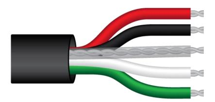
Red: Power In (4.5 to 24 V DC) Black: SDI-12 Data Line Clear: Ground (shield wire) White: Positive Heater Power Green: Negative Heater Power
