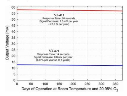
Long-term stability (output voltage decrease over time) of Apogee SO-400 series oxygen sensors. The response time and signal decrease for both series are also listed.
