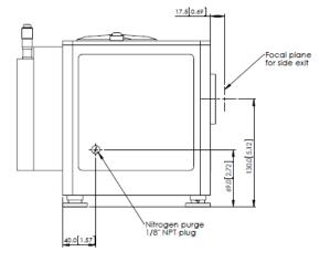
Standard configuration shown with manual slit on input, CCD flange on straight output.
