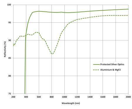
The graph shows the standard AI + MgF<sub>2</sub> optics coatings reflection efficiency versus wavelength.
