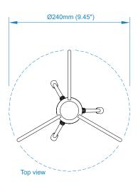
Positions for three off bolt fixings with Ø7.0mm (0.27") max. thread. on a p.c.d. of 85mm (3.35")
