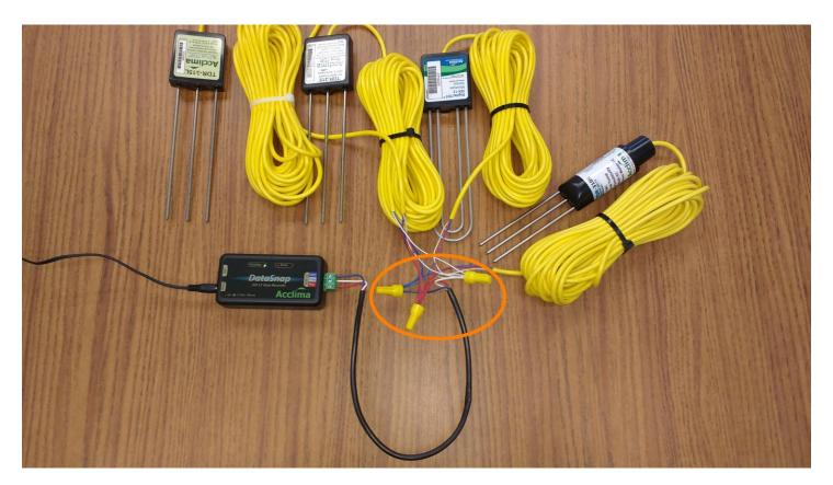
Figure 7 – Extended wiring splice example
