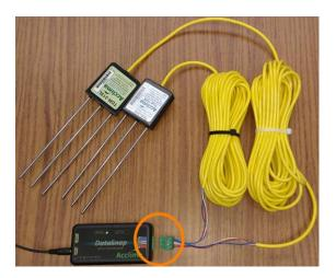
Figure 6 – Terminal Block Plug-in
