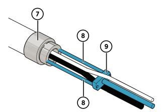
Figure 5 Supporting HMT330WPA with a Threaded Bar
