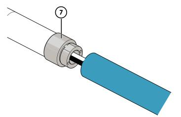
Figure 4 Supporting HMT330WPA with a Cable Conduit
