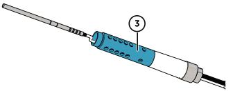
4. Insert the grommet (1) to the hole at the end of the T measuring tube (2). Then push the temperature probe through the grommet and tighten the tube.
