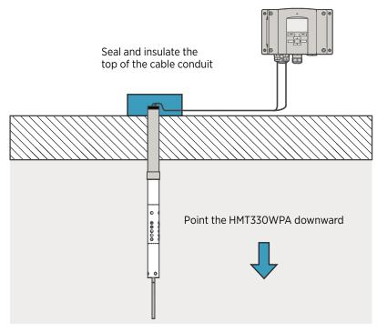
Figure 1 Recommended Installation using a Cable Conduit
