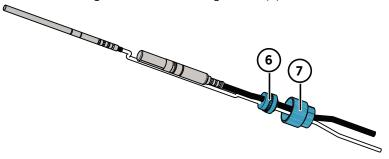
2. Insert the first tube (5) over the probes and tighten it to the screw sleeve (7). Insert the small white plastic support (4) to the cable at the base of the RH measurement probe. Route the cable of the T probe so it rests in the cutout of the support. Push the screw sleeve so that the support goes inside the tube.
