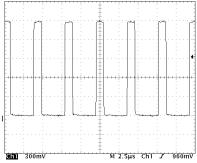
244KHz Frequency, 1500V Output 2.5us/Div horizontal scale, 300V/Div vertical scale)
